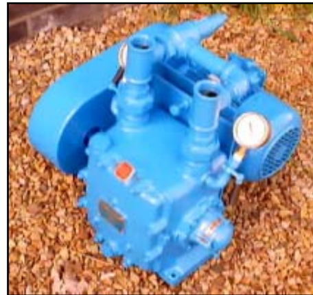
📍 L125V Bilge pump
