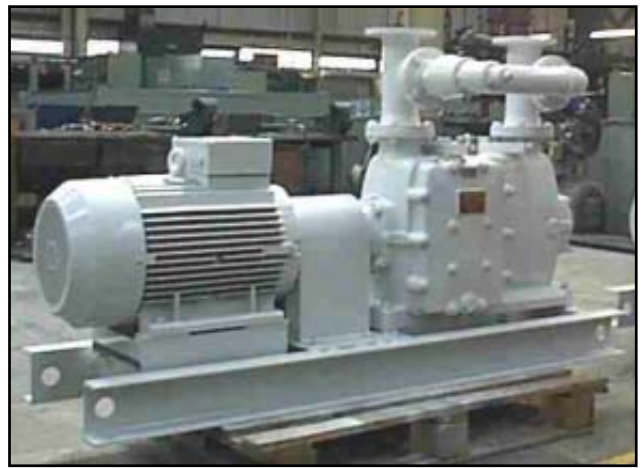
🔦 L400 bronze bilge pump, 50m 3 /hr capacity
